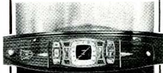
STUDEBAKER provides a dummy glove compartment plate, at the left, for dials. Radio is "extra"
